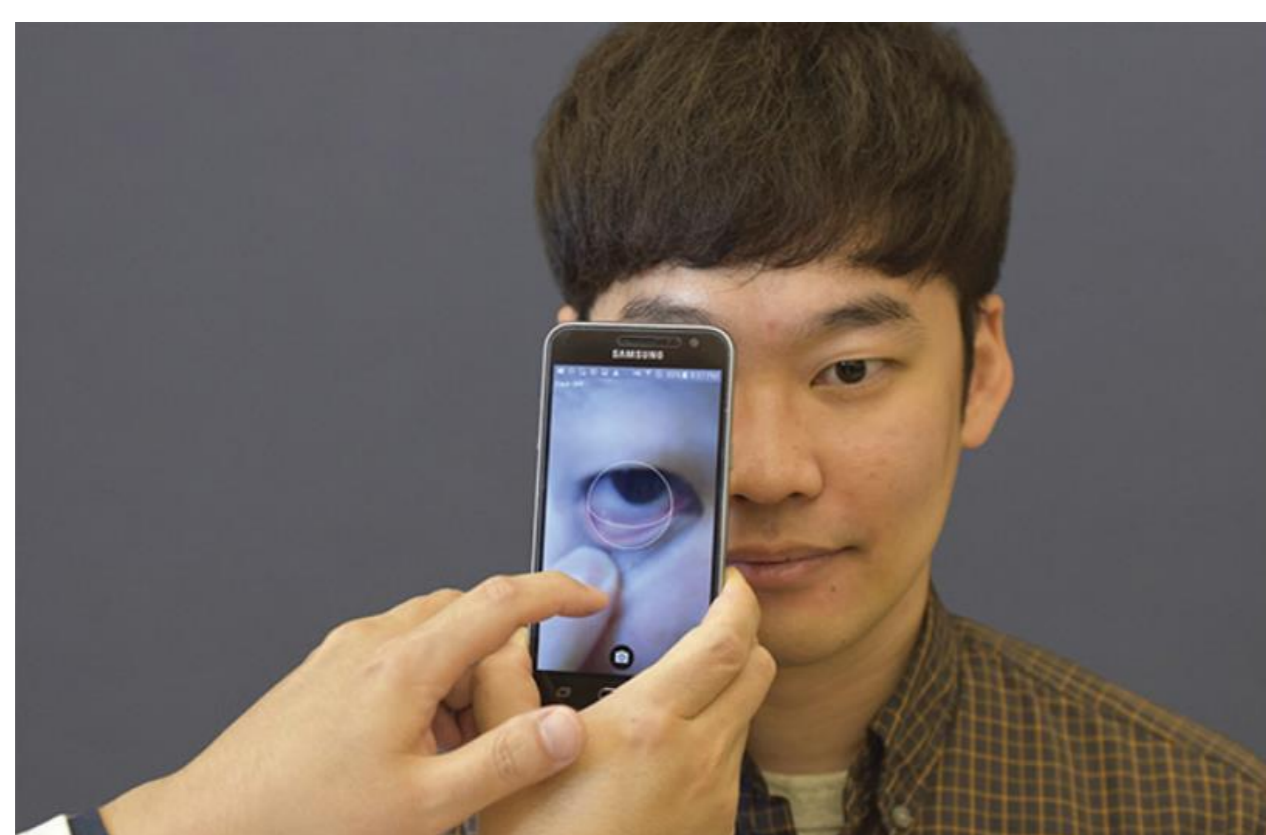
Figure 2. The mobile application for noninvasive blood hemoglobin quantification.
